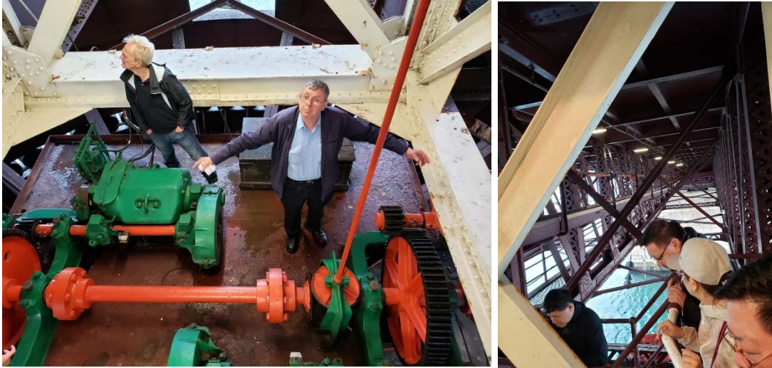
The open span was lifted up and the open span is rotated by 60 large steel wheel at the turn table.
