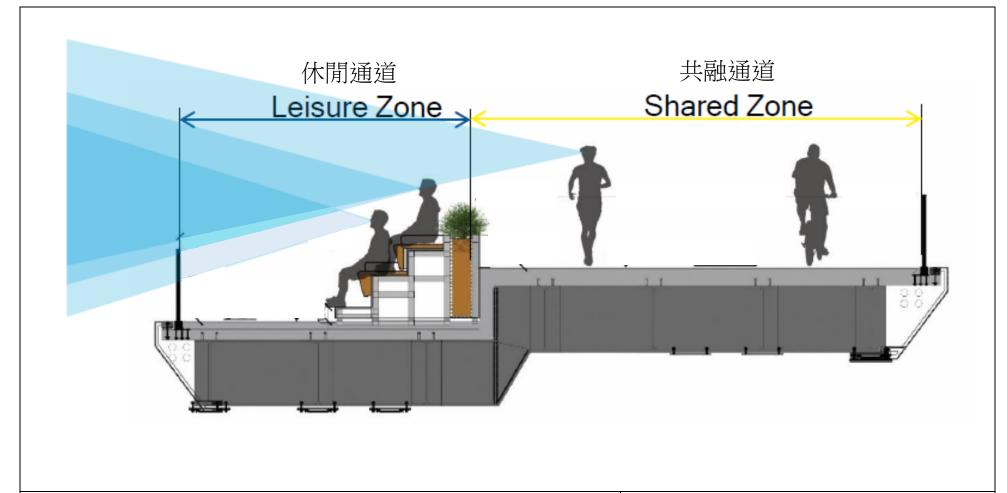
東區走廊下之行人板道 – 梯級式座位切面圖 Boardwalk underneath Island Eastern Corridor – Typical Section of Cascade Seating
